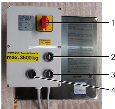
Operating element with internal hydraulic unit and CE Stop button
