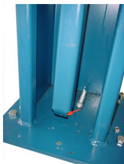
Pic 6: Hang the spring into the ratchet-strip
