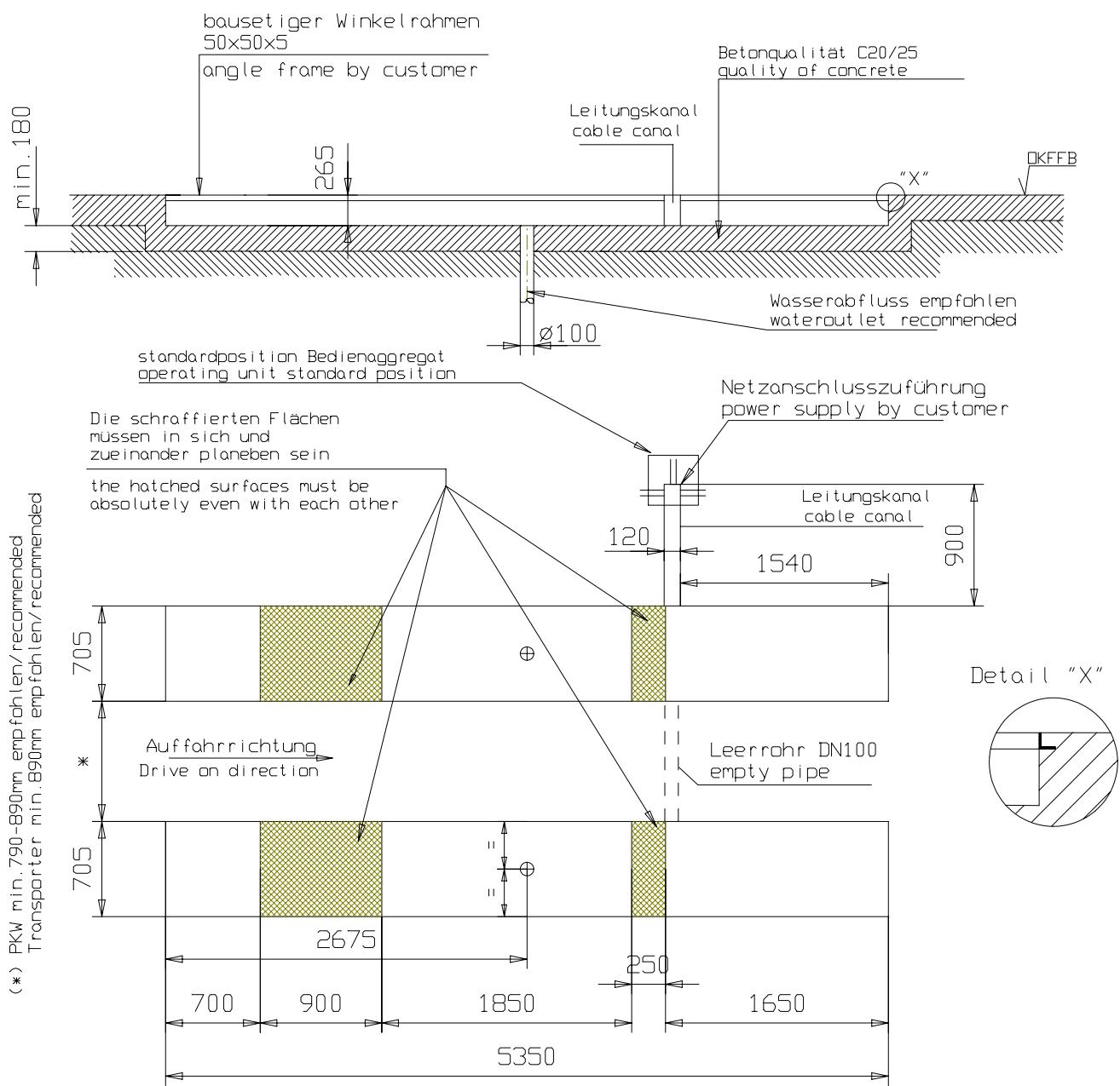
Valid for the standard inground version of the lift with drive-on ramp at each side of the platform. Instead of the cable duct a empty pipe with 100mm diameter can be used to lead the hoses and cables to the operating unit. If desired the position of the power unit can be changed. If necessary adapt the supply lines.
